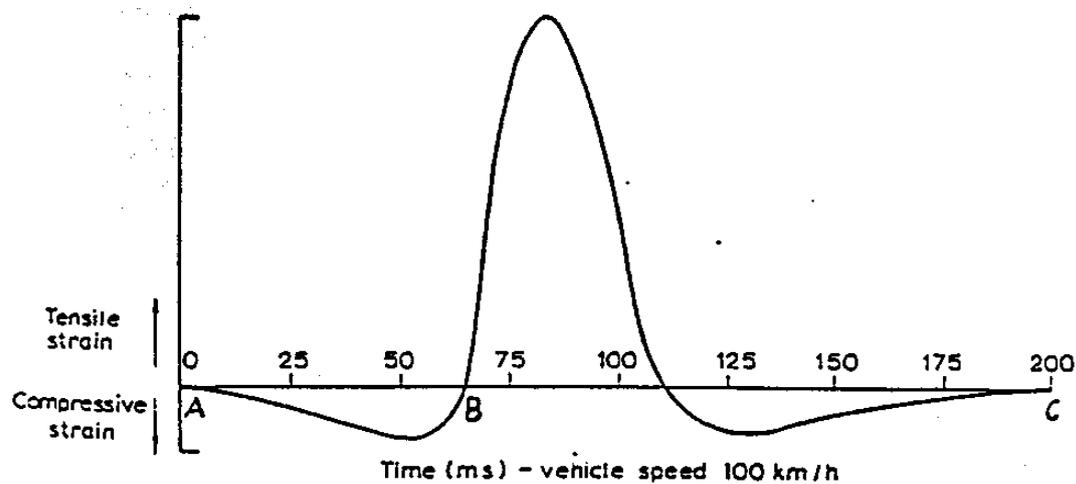
**Figure 3: Typical Longitudinal Strain Profile for Moving Wheel (100 km/h)**
