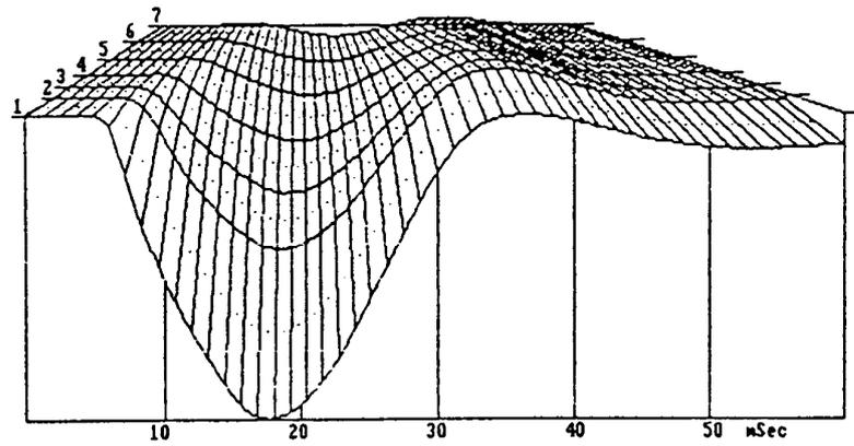
**Figure 4: Deflection Response of FWD Load Pulse**
