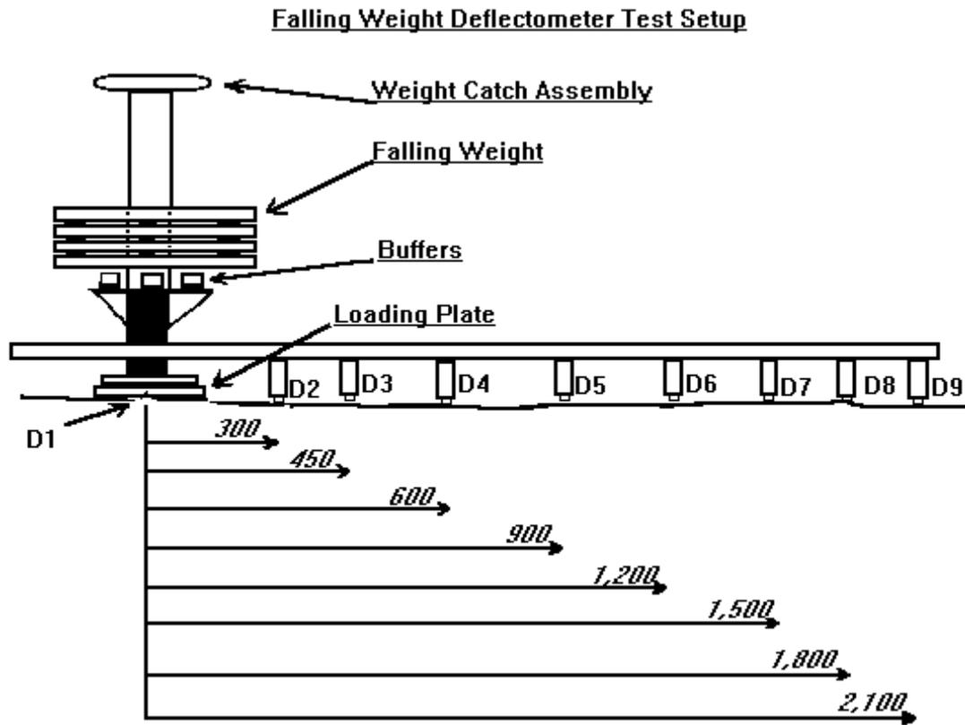
**Figure 2: Diagrammatic Representation of FWD**
