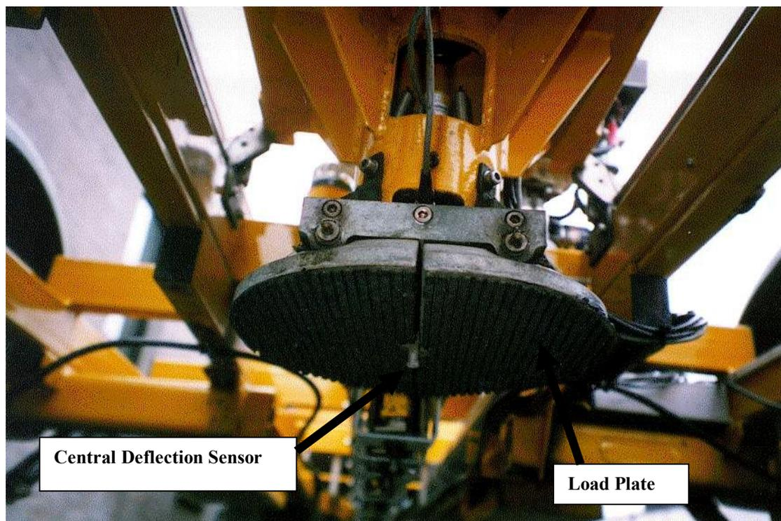
**Figure 1: Segmented FWD Load Plate**
