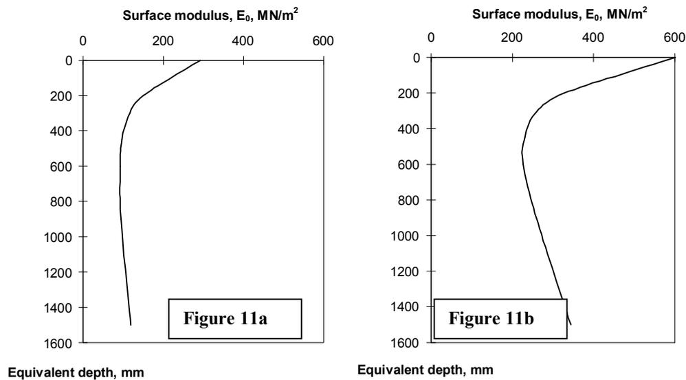
**Figure 11a,b. Examples of surface moduli plots.**
