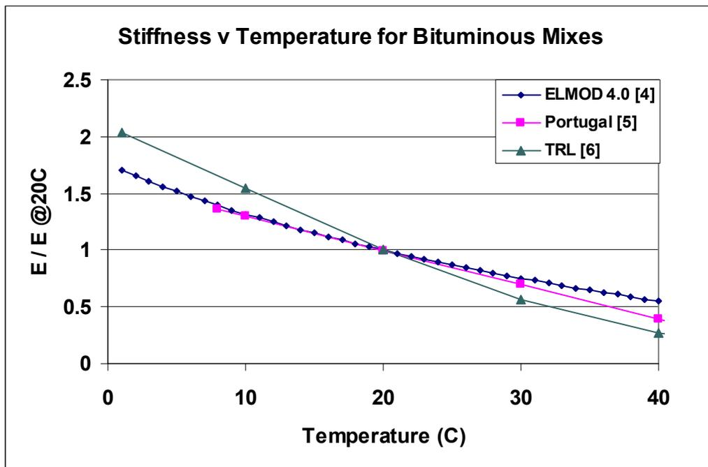
**Figure 13: Stiffness versus Temperature relationships**
