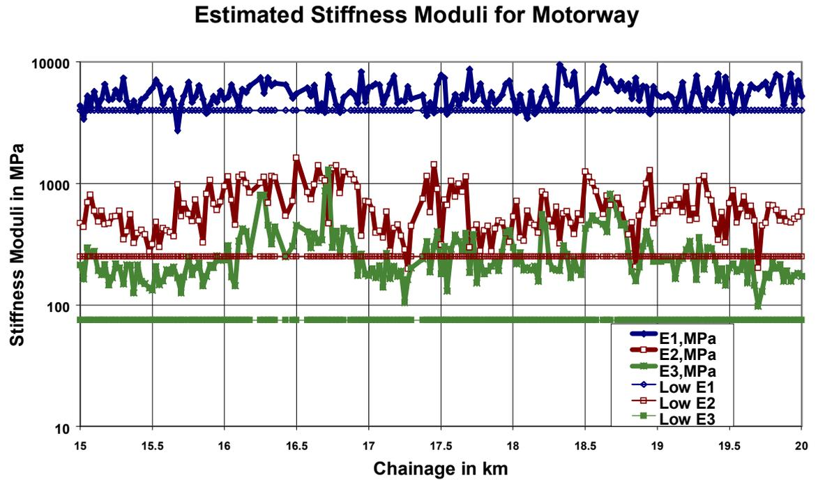
**Figure 14: Estimated Stiffness Values for Motorway<sup>(4)</sup>**
