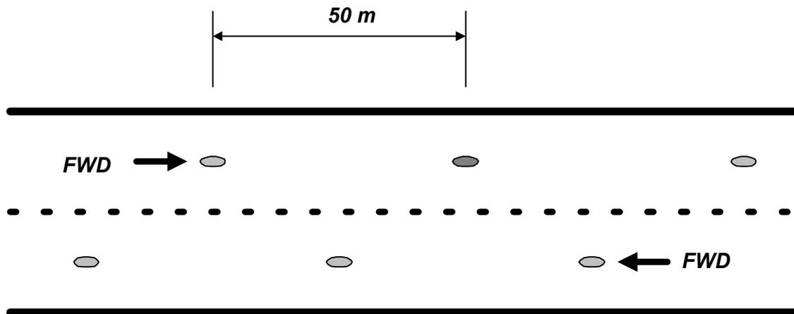
**Figure 8: Staggered FWD test points on two lane road**
