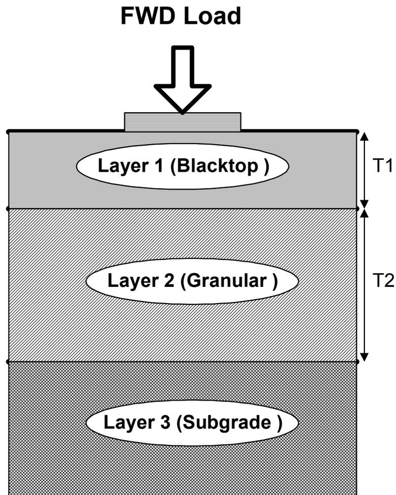
**Figure 12: Three Layer Pavement Model**
