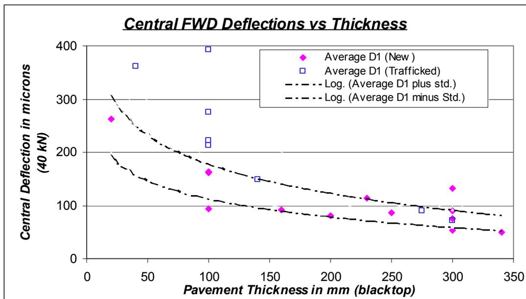
Figure 10: Plot of central deflections versus Blacktop thickness
