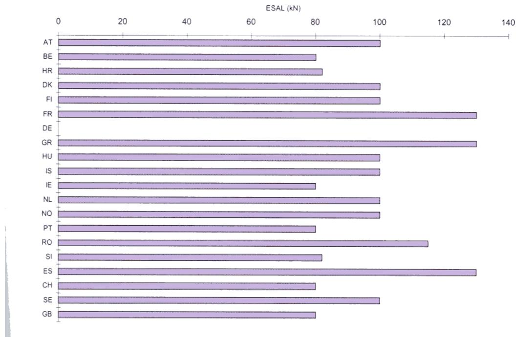
**Figure 5: Design Axle Loads Used in Europe<sup>(3)</sup>**
