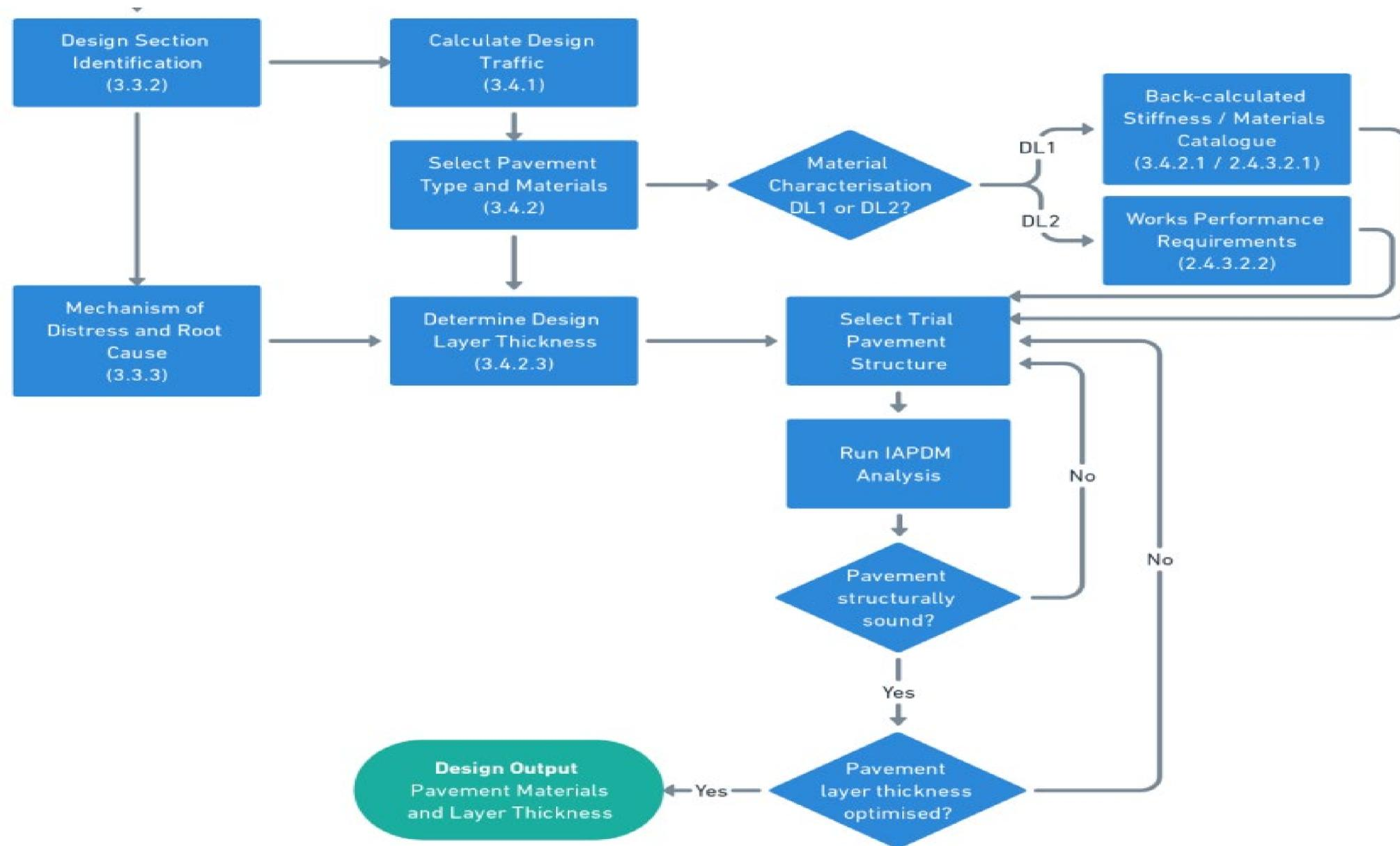
Figure 3.1 Existing Pavement Assessment and Maintenance Intervention Design Process
