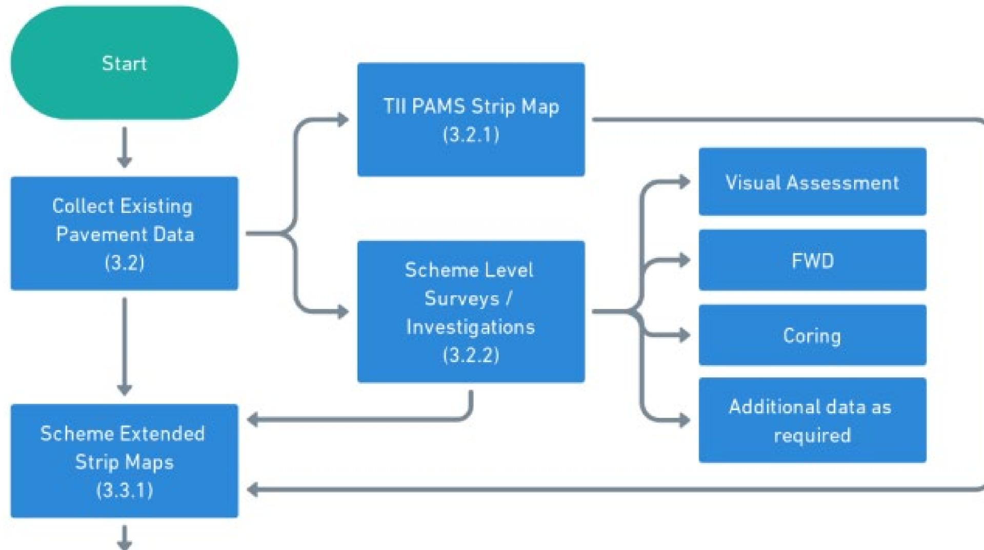
**Figure 3.1 Existing Pavement Assessment and Maintenance Intervention Design Process**
