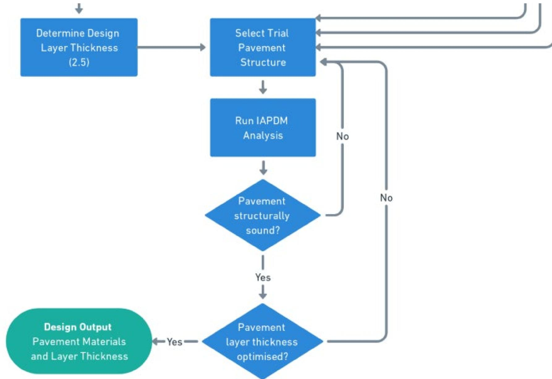
**Figure 2.1 New Pavement Design Process**
