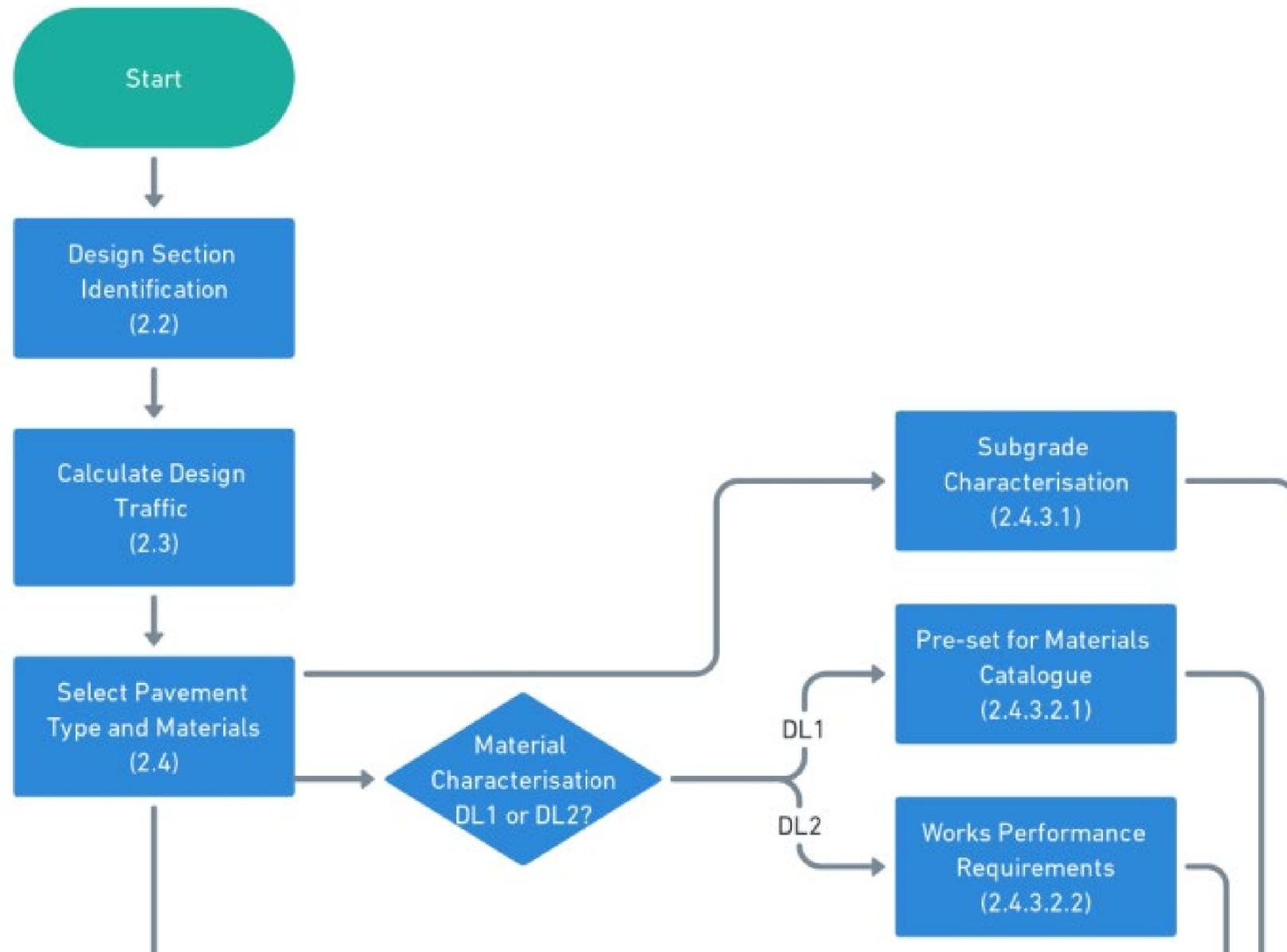
**Figure 2.1** New Pavement Design Process
