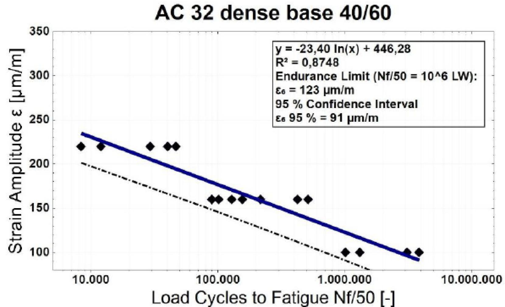
**Figure 11: Fatigue results of AC 32 dense base 40/60**
