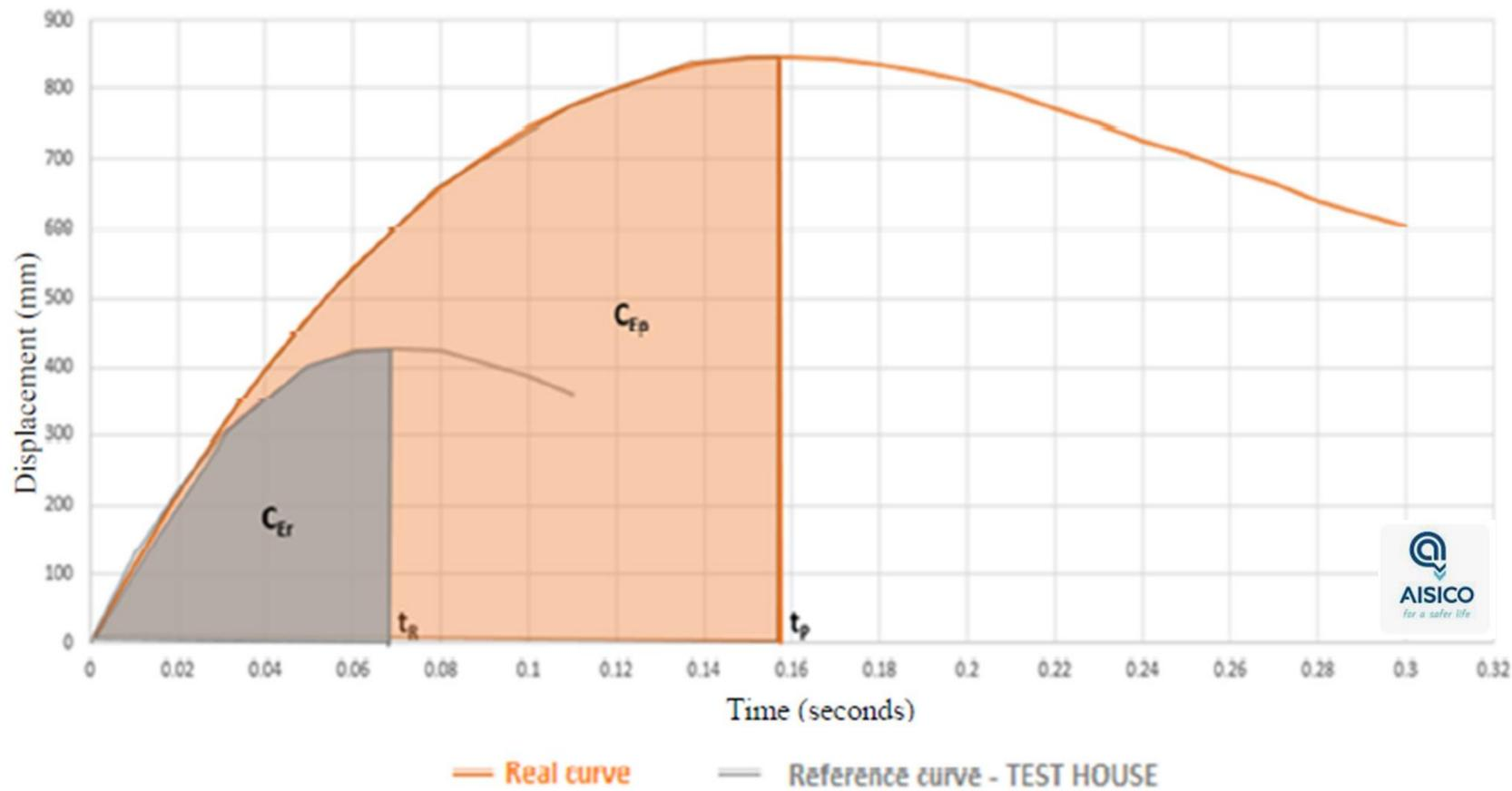
Displacement vs. time curve derived from the dynamic test
