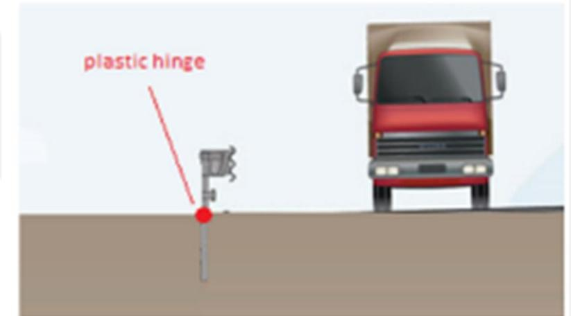
Plastic hinge develops at ground level or higher.
