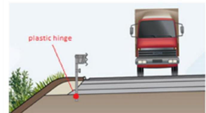
Plastic hinge may not develop at all or may occur at a lower level than required by the design.
